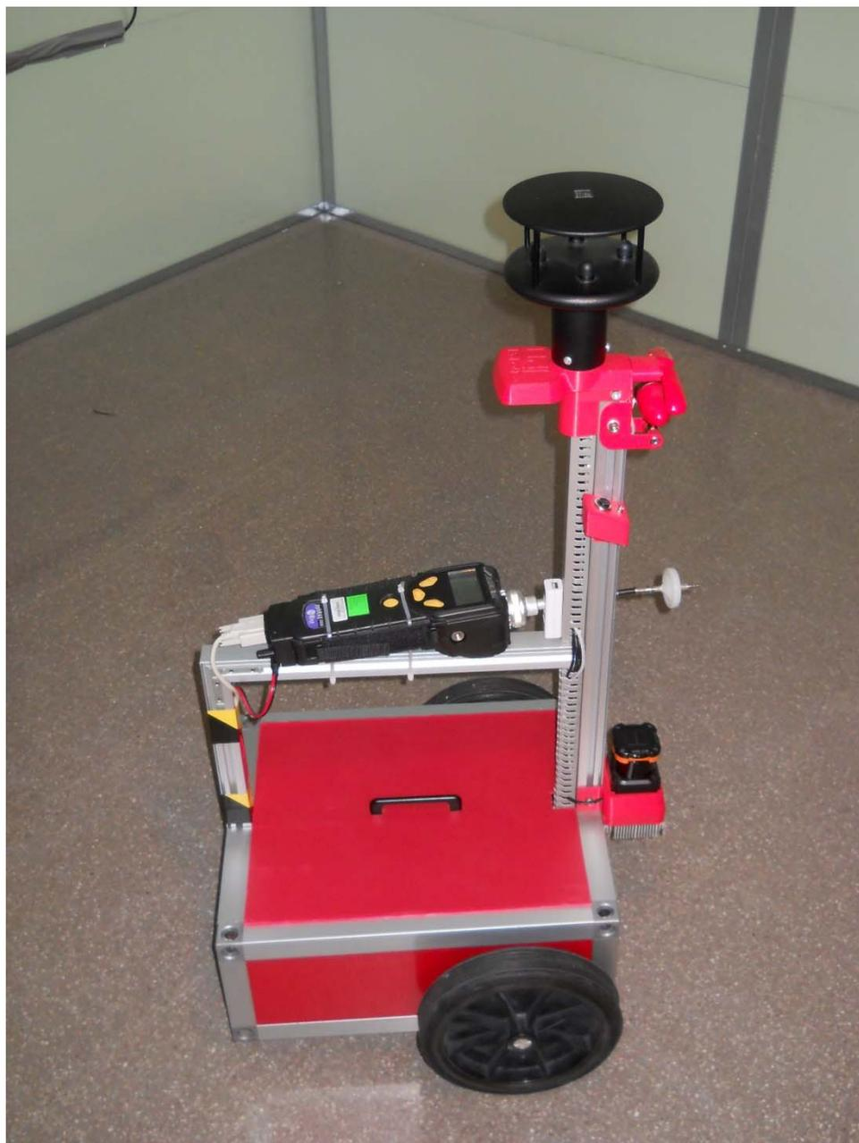
**Figure S3.** Autonomous robot featuring the wind sensor and the photoionization detector.
