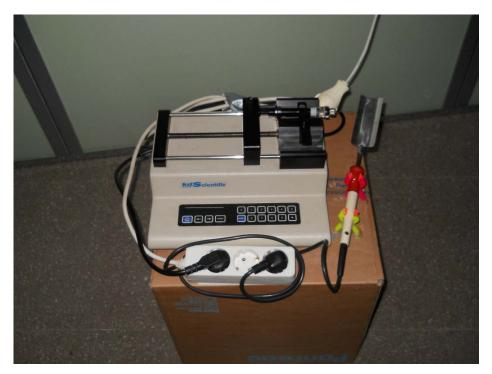
**Figure S2.** Chemical delivery system based on a KDS-200 injection pump. Drops fall in a hot plate for immediate vaporization.
