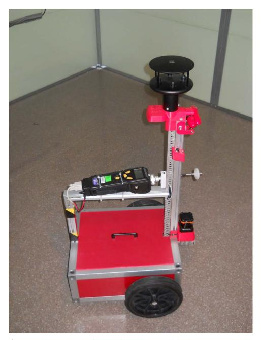
**Figure S3.** Autonomous robot featuring the wind sensor and the photoionization detector.
