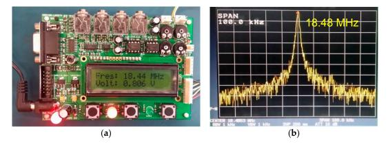
**Figure 10.** The test results of the portable spectrum analyzer and the spectrum analyzer R3272: (a) The result obtained by the portable spectrum analyzer; (b) The result obtained by the spectrum analyzer R3272.
