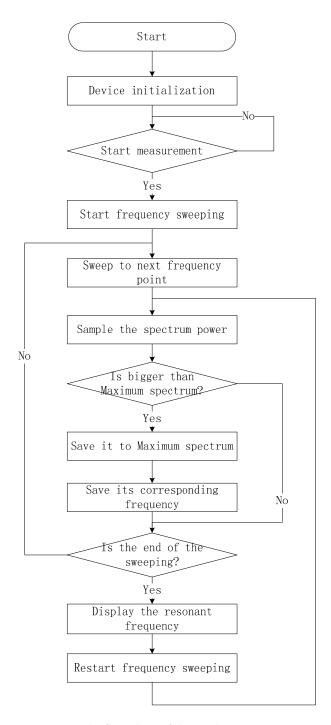
Figure 6. The flow chart of the geodetic strainmeter.
