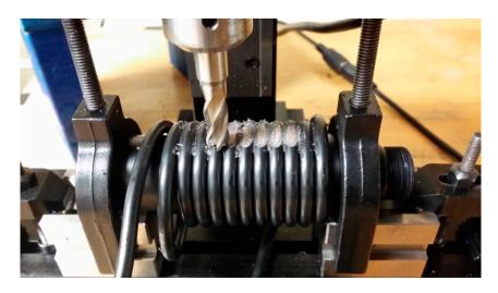
Figure 7. The CCBG produced on a milling machine.
