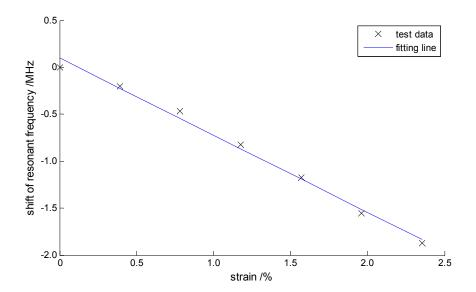
Figure 12. The test results of the axially tensile strain.
