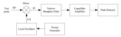
Figure 3. The block diagram of a spectrum analyzer based on the Heterodyne principle.
