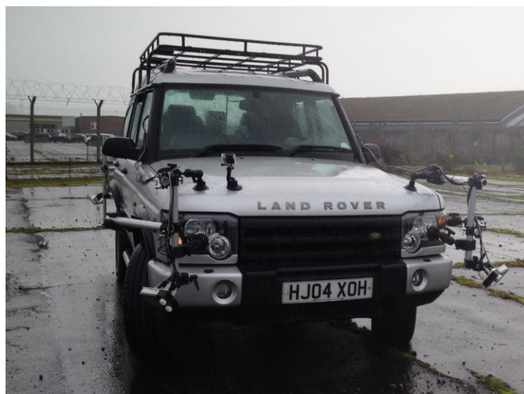
Figure 6. (a) A 4-radar Janus configuration. Top and side view of the test vehicle showing the depression and azimuth angle of the radar sensors; (b) A 4-radar Janus configuration. An actual image of the test vehicle with radars and a video camera installed.
