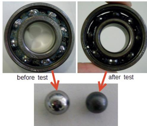
Figure 8. Bearing before and after test.
