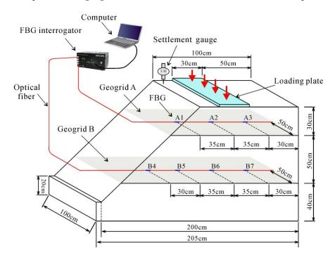
**Figure 1.** General arrangement of the geogrid-reinforced slope and locations of fiber Bragg grating (FBG) sensors.
