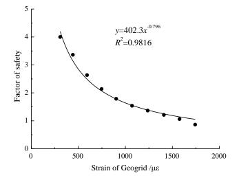
Figure 9. Relationships between the factor of safety and geogrid characteristic strain.
