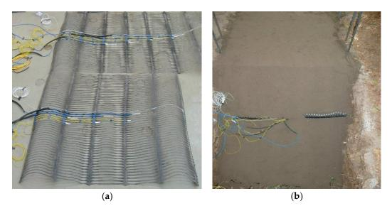
**Figure 2.** Photographs of the geogrid and **s**lope model: (**a**) geogrid installed with sensors; (**b**) upward view of the slope.
