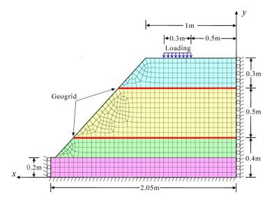
Figure 3. Finite element model.
