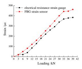
Figure 4. Comparison between FBG and electrical resistance strain gauge test results.
