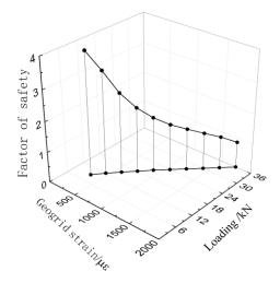
Figure 10. Relationship between loading, characteristic maximum strain, and the factor of safety.
