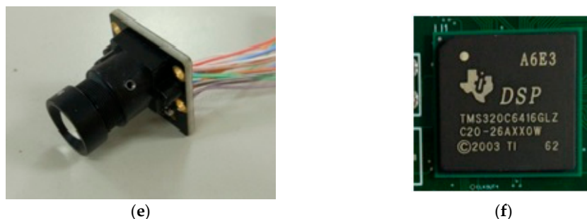
Figure 17. (a) the swing table; (b) turntable; (c) the pattern picture pasted on the swing table; (d) position of each part; (e) the camera; (f) the DSP chip C64XX.
