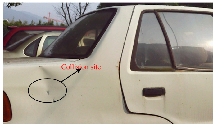
Figure 5. Deformation caused by a real accident.
