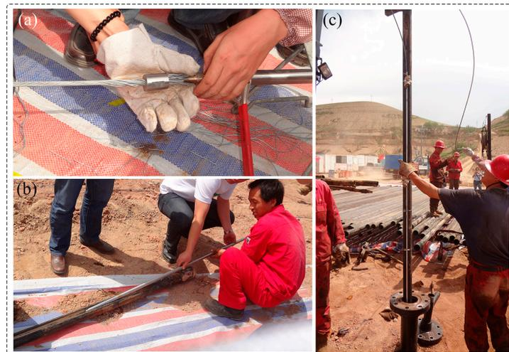
**Figure 22.** Photos of well-logging field: (a) Downhole cable; (b) Tied to the downhole tube; (c) Sensor down well process.
