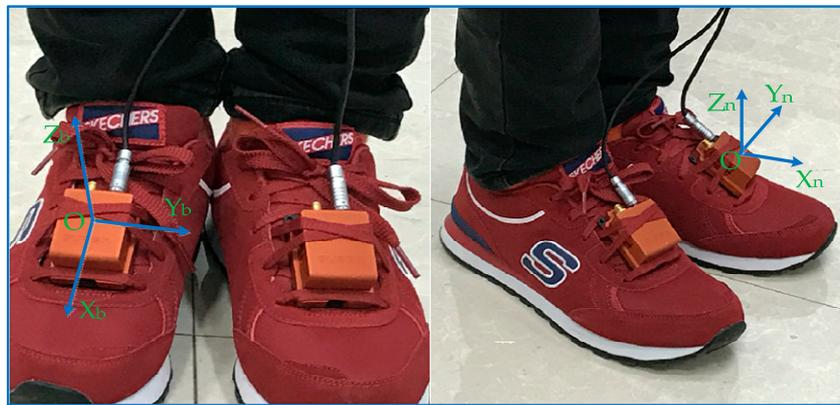
**Figure 1.** (Left) The two MIMU are mounted to the feet separately, the  $OX_bY_bZ_b$  coordinate system are the carrier coordinates; (right) side view, the  $OX_nY_nZ_n$  coordinate system are the navigation coordinates.
