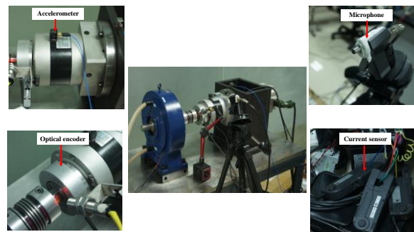
Figure 5. Four types of sensors and their installations.
