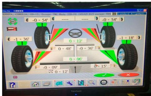
**Figure 9.** The camber measuring results from a traditional vision-based system.
