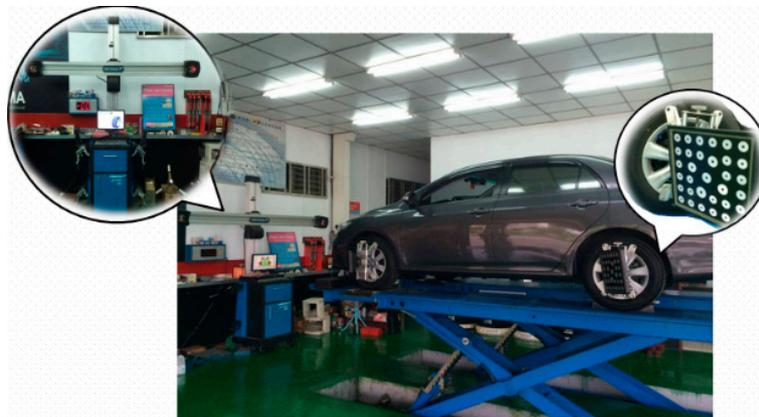
**Figure 1.** A typical computer vision-based inspection system for wheel alignments.
