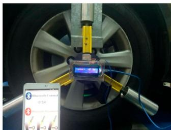
**Figure 10.** The result evaluated camber angle from the MUC-based system for the front-right wheel of a vehicle.
