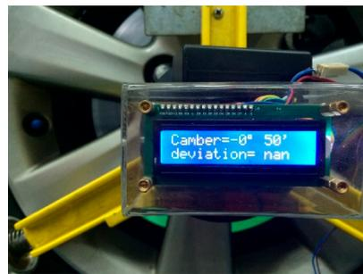
**Figure 7.** The MCU-based camber inspection system.
