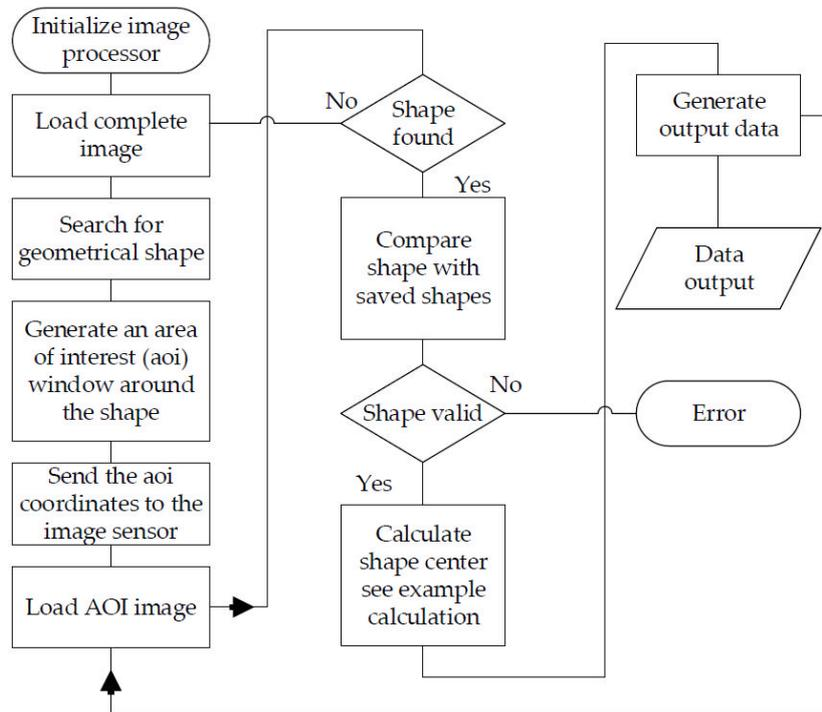
Figure 9. Schematic software procedure—normal use.
