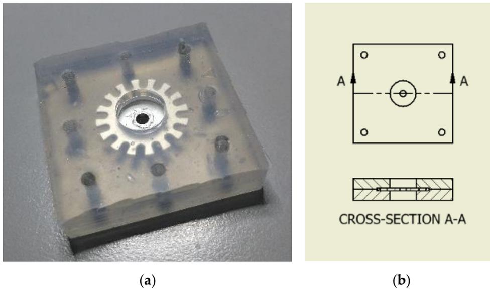
**Figure 4.** (a) Polymer with encapsulated movement carrier, encapsulated version 1 (b) Polymer with movement carrier, cross-section, version 1.
