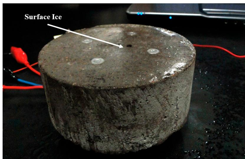
Figure 8. Surface ice formation on cold SP-I sensor.
