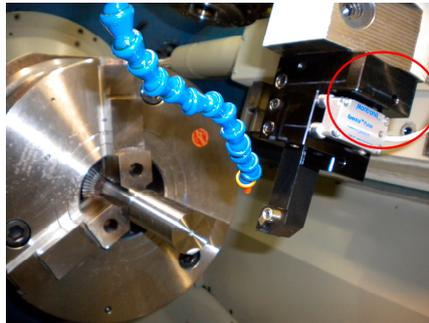
Figure 1. Three-axis vibration sensor mounted on the tool holder.
