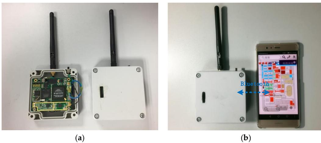
Figure 16. The positioning receiver: (a) is the internal and external structure of the receiver, and (b) shows that the receiver uploads the related data to the mobile phone through Bluetooth to display.
