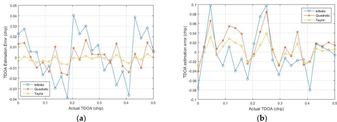
**Figure 13.** The time difference of arrival (TDOA) estimation errors under different setting code phase differences: (a) is SNR = 0 dB and (b) is SNR =  $-15$  dB.
