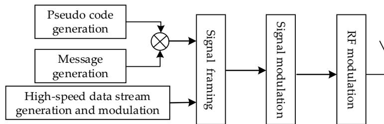
**Figure 2.** Flowchart of the signal generation.
