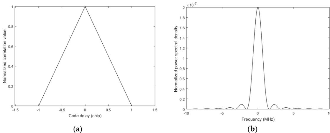
**Figure 4.** Characteristics of the autocorrelation function: (a) is autocorrelation function with infinite bandwidth; and (b) is power spectral density.
