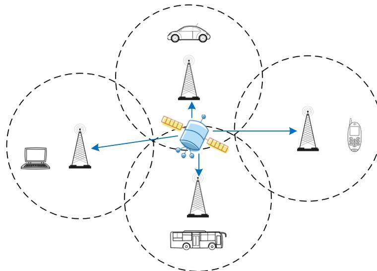
**Figure 1.** Terrestrial single frequency network coverage of the China mobile multimedia broadcasting (CMMB) system.
