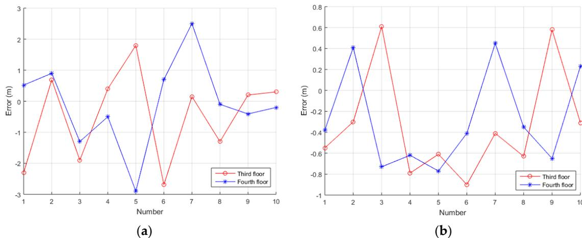
**Figure 20.** The positioning accuracy of the entire system: (a) is horizontal accuracy and (b) is vertical accuracy.
