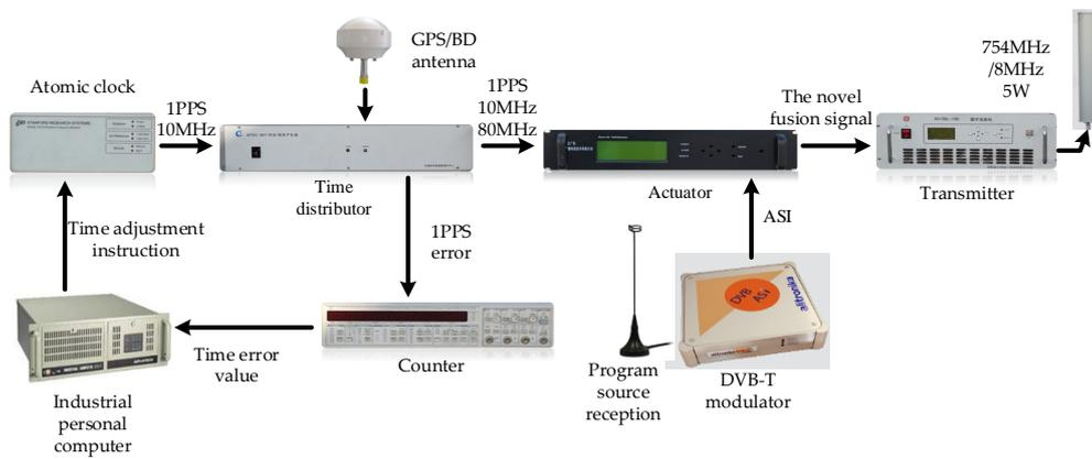
Figure 15. Each equipment of the modified base station.
