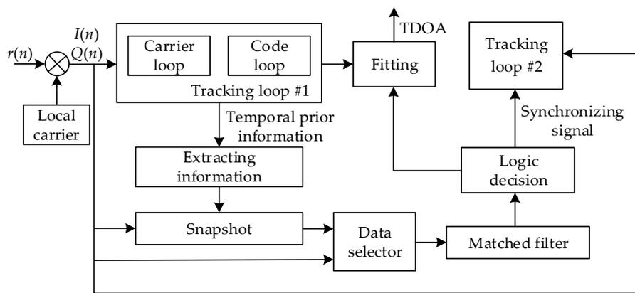
Figure 7. Flowchart of the proposed algorithm.
