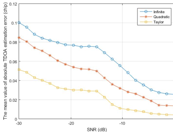
**Figure 14.** The TDOA estimation errors under different signal-to-noise ratio (SNR).
