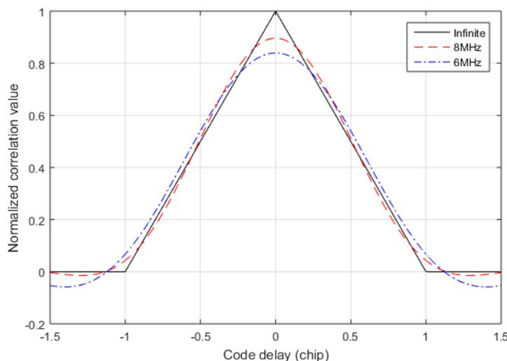
Figure 6. The autocorrelation function under different bandwidths.
