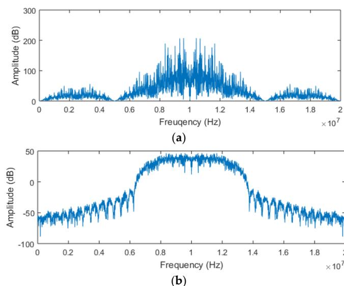
**Figure 12.** The spectrum of received signals: (a) is before filtering and (b) is after filtering.
