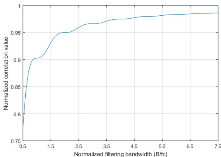
**Figure 5.** The proportion of the signal component through the filter in the total signal under different bandwidths.
