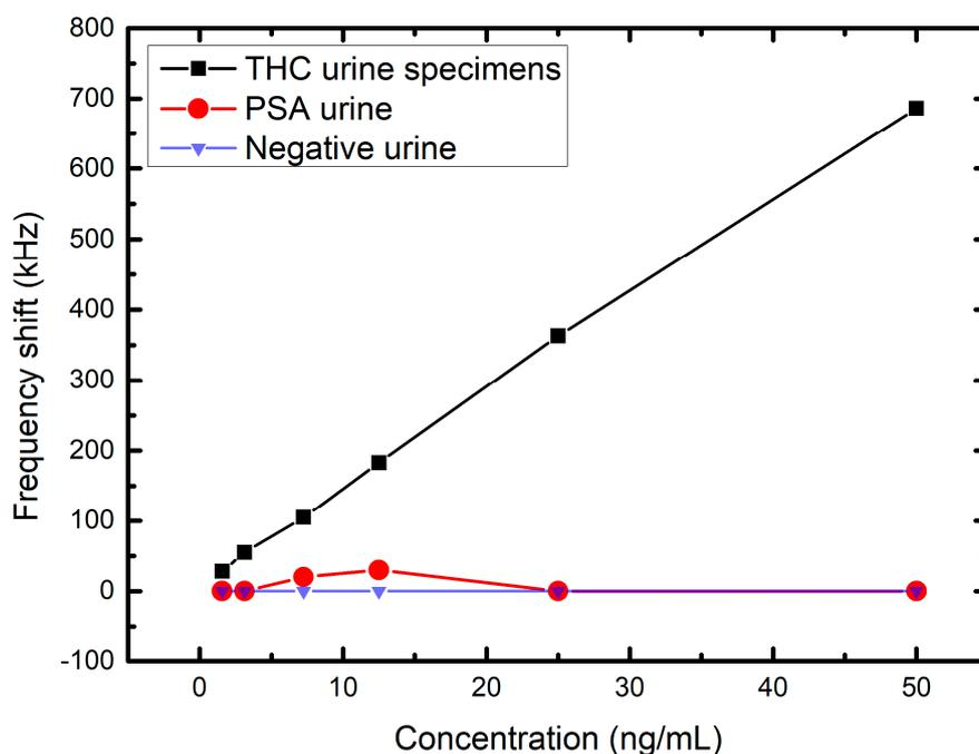
Figure 9. Measurement results of the THC urine specimens, PSA urine, and negative urine.
