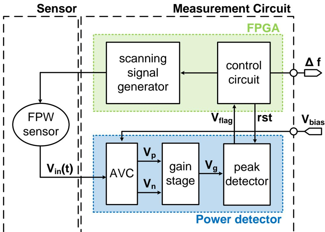
Figure 3. Block diagram of the FPW readout system.
