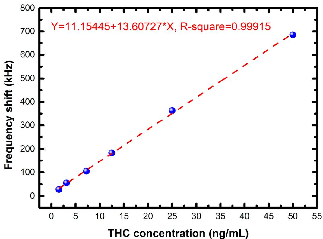
Figure 8. Measurement results of the FPW readout system prototype.
