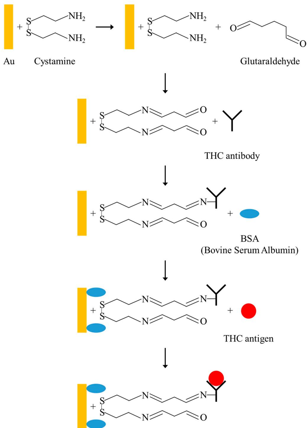
**Figure 2.** Schematic diagram for the integration of cystamine SAM, glutaraldehyde, THC antibody, and THC antigen in multilayers.
