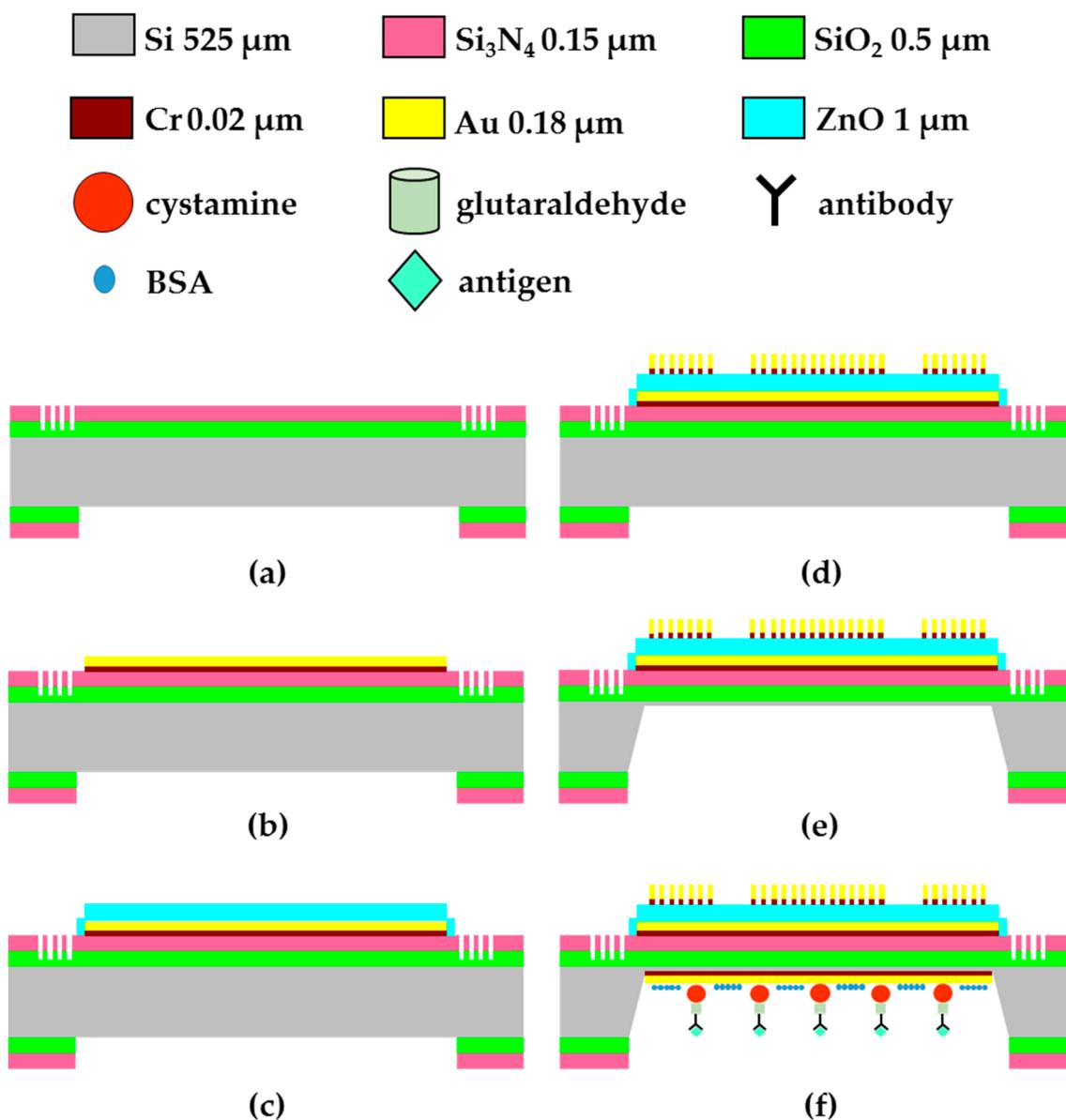
**Figure 1.** Main processing steps of the proposed FPW device: (a) deposit  $\text{SiO}_2/\text{Si}_3\text{N}_4$ , etch Si-groove RGS, and pattern backside  $\text{SiO}_2/\text{Si}_3\text{N}_4$ ; (b) deposit and pattern Cr/Au ground electrode; (c) deposit and pattern ZnO; (d) deposit and pattern Cr/Au IDTs; (e) etch the backside silicon by using 30 wt % KOH at 60 °C and 30 wt % KOH at 27 °C; (f) the THC antibody has to be coated on the back-side silicon cavity to catch the THC antigen in urine.
