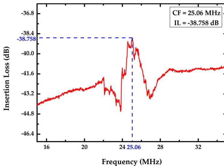
Figure 5. Frequency responses of the proposed FPW device.
