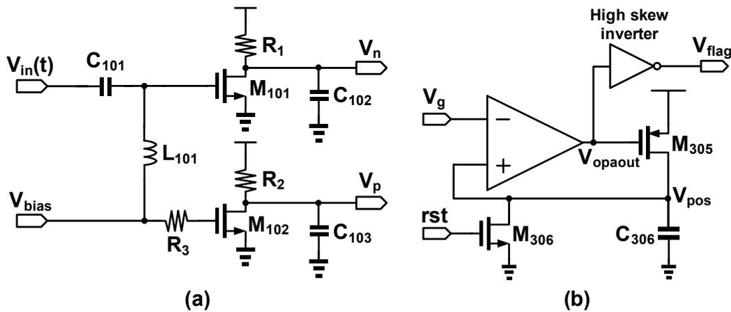
Figure 4. Schematic of (a) amplitude-to-voltage converter (AVC) and (b) peak detector.
