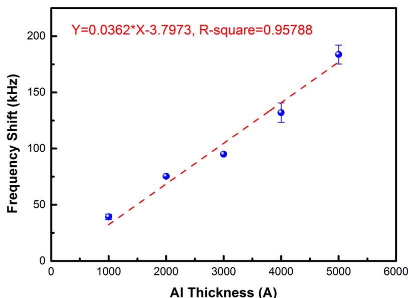
**Figure 6.** The frequency shifts of the FPW device with five different Al mass loadings.
