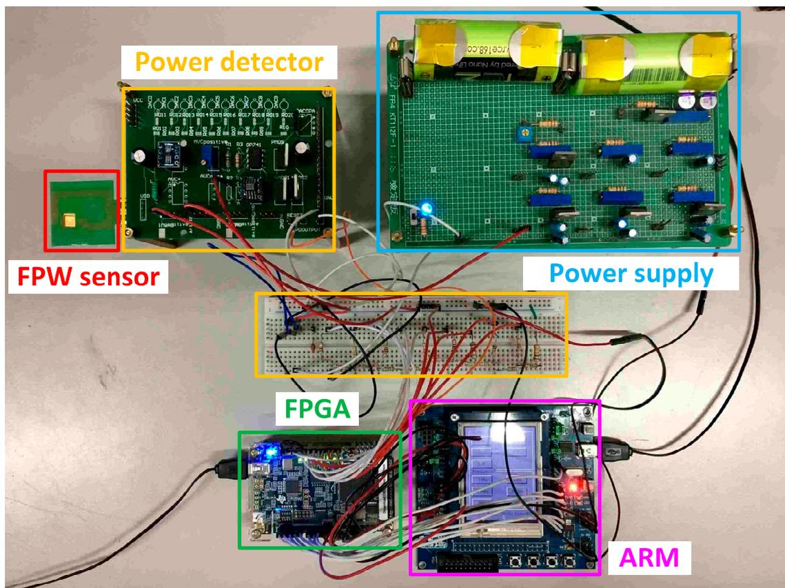
Figure 7. Photo of the system prototype measurement environment.
