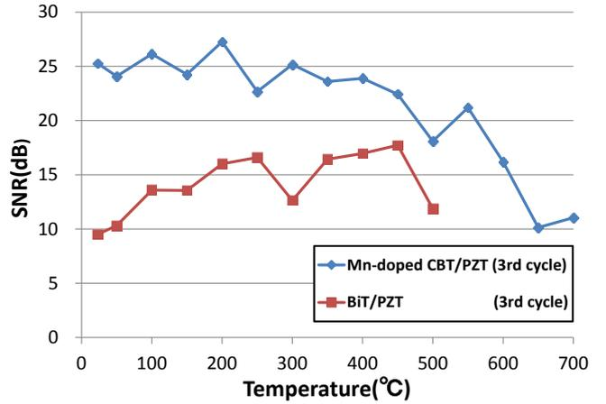
Fig. 7. Temperature dependency of SNR for Mn-doped CBT/PZT and BiT/PZT in 3<sup>rd</sup> cycle.
