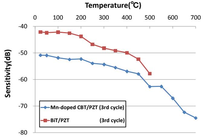
Fig. 6. Temperature dependency of sensitivity for Mn-doped CBT/PZT and BiT/PZT in 3<sup>rd</sup> cycle.
