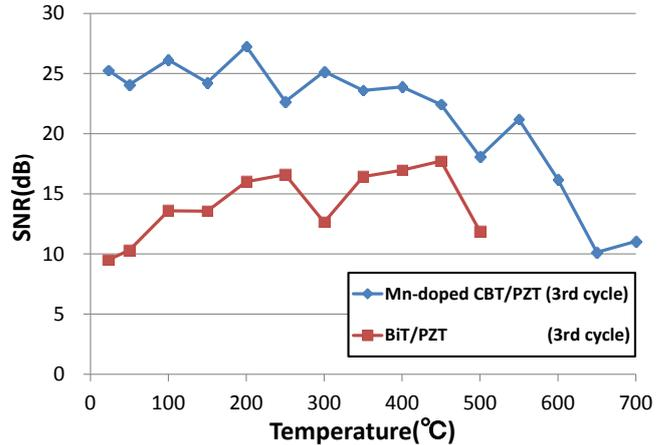
Fig. 7. Temperature dependency of SNR for Mn-doped CBT/PZT and BiT/PZT in 3rd cycle.
