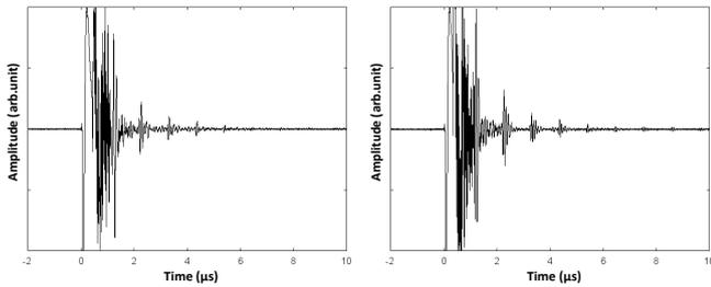
Fig. 9. Ultrasonic responses of BiT/PZT at 500°C after (a) 0h and (b) 36 h.
