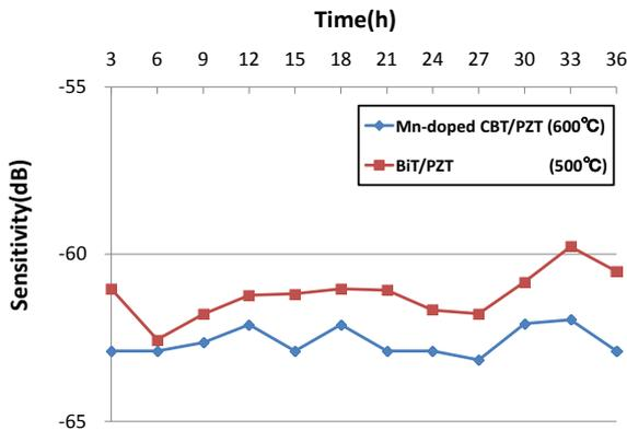
Fig. 10. Comparison of SNR of Mn-doped CBT/PZT and BiT/PZT in 3rd cycle.
