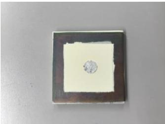
Fig. 2. Optical images of BiT/PZT films fabricated onto 3.3 mm thickness, ~30 mm length, and ~30 mm width titanium substrate.
