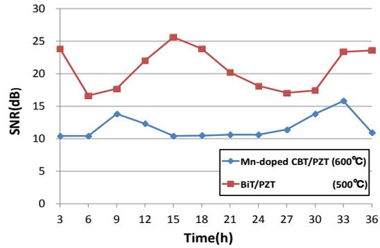
Fig. 11. Time dependence of SNR of Mn-doped CBT/PZT and BiT/PZT during 36h.
