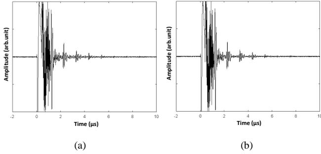
Fig. 5. Ultrasonic responses of BiT/PZT at 500°C in (a) 2<sup>nd</sup> thermal cycle and (b) 3<sup>rd</sup> thermal cycle.
