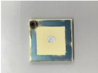
Fig. 1. Optical images of Mn-doped CBT/PZT films fabricated onto 3.3 mm thickness, ~30 mm length, and ~30 mm width titanium substrate.
