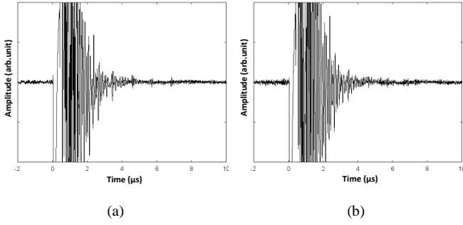
Fig. 4. Ultrasonic responses of Mn-doped CBT/PZT at 700°C in (a) 2<sup>nd</sup> thermal cycle and (b) 3<sup>rd</sup> thermal cycle.
