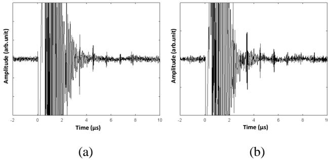
Fig. 8. Ultrasonic responses of Mn-doped CBT/PZT at 600°C after (a) 0h and (b) 36 h.
