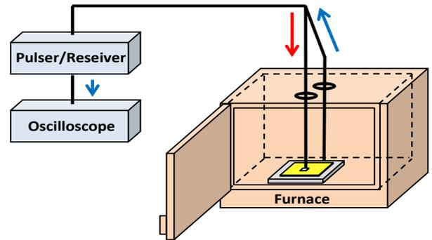
Fig. 3. Schematic diagram for ultrasonic measurement at high temperatures.
