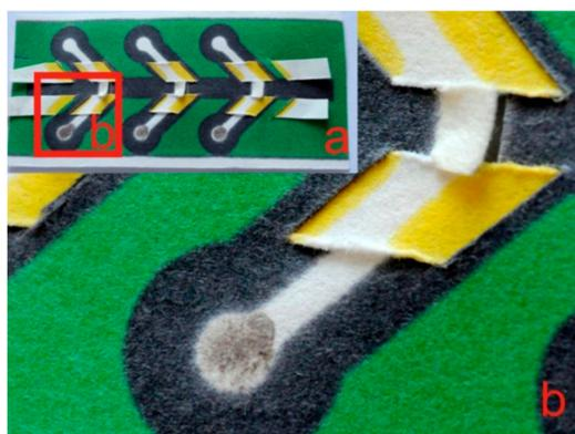
**Figure 14.** (a) The photograph of the switch-on-chip and (b) the enlarged view of the inlet and the pretreatment zone [139].
