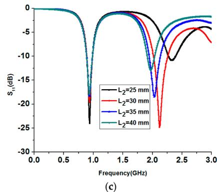
**Figure 3.** (a) Parametric study for  $L_5$  in the unfolded state; (b) parametric study for length of the stub ( $L_1$ ); (c) parametric study for position of stub ( $L_2$ ).
