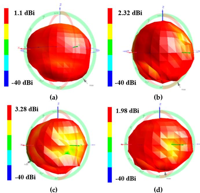
**Figure 5.** Measured 3D radiation patterns of the proposed origami magic cube antenna in the unfolded state (a,b): (a) at 900 MHz, (b) 2200 MHz; measured 3D radiation patterns of the proposed origami magic cube antenna in the folded state (c,d): (c) 1500 MHz, (d) 2400 MHz.
