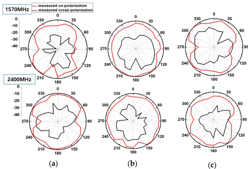
**Figure 7.** Measured 2D normalized radiation patterns of the proposed origami magic cube antenna in the folded state. (a) yz-plane, (b) xz-plane, (c) xy plane.
