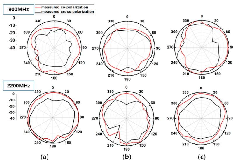
**Figure 6.** Measured 2D normalized radiation patterns of the proposed origami magic cube antenna in the unfolded state. (a) yz-plane, (b) xz-plane, (c) xy-plane.
