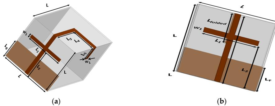
**Figure 1.** Proposed origami magic cube antenna (a) in the unfolded state (b) magic cube antenna in the folded state ( $L = 50 \text{ mm}$ ,  $L_1 = 24 \text{ mm}$ ,  $L_g = 20 \text{ mm}$ ,  $L_2 = 30 \text{ mm}$ ,  $L_3 = L_4 = 25 \text{ mm}$ ,  $L_5 = 15 \text{ mm}$ ,  $W_1 = 2 \text{ mm}$ , and  $L_{\text{folded}} = 25 \text{ mm}$ ).
