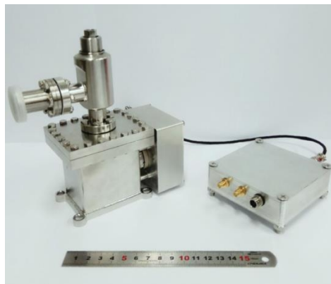
Figure 7. The prototype of the accelerometer. The spring-mass structure is encapsulated in a small vacuum cavity (left) and the circuit is installed in a shielding box (right).
