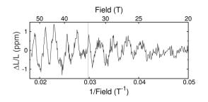
**Figure 7.** Magnetostrictive quantum oscillations in GdSb at 2 K taken in a 55 T mid-pulse magnet using the method described in Section 2.2. The resolution achieved in this measurement is considerably better than  $10^{-6}$  [9].
