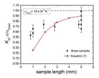
**Figure 14.** Strain transfer coefficient computed using Equation (7) (red circles), and measured coefficient of thermal expansion divided by  $\alpha_{\text{brass}} = 19 \text{ ppm/K}$  (black squares). The analytic solution fails to reproduce the experimental data in the 1 mm-long sample limit.
