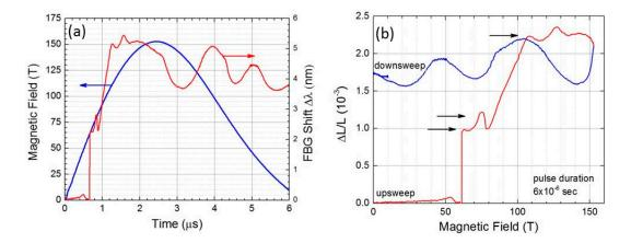
**Figure 8.** Axial magnetostriction obtained in a destructive 6 microsecond single-turn coil type magnet, figure reproduced from [17]. (**a**). Magnetic field (left y-axis, blue line) and FBG shift (right y-axis, red line) vs. time. (**b**). Computed  $\Delta L/L$  vs. magnetic field for magnetic field upsweep (red) and down sweep (blue). Spin transitions at 60 T and 75 T, as well as a previously unknown transition at ~106 T, are indicated by arrows.
