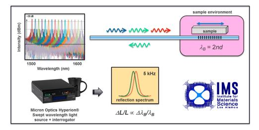
**Figure 2.** Experimental setup for fiber Bragg gratings (FBG) interrogation with a swept wavelength laser source, such as the Micron Optics Hyperion<sup>®</sup> instrument.  $\lambda_B$  is the Bragg wavelength, *n* is the fiber's index of diffraction, and *d* is the grating spacing.
