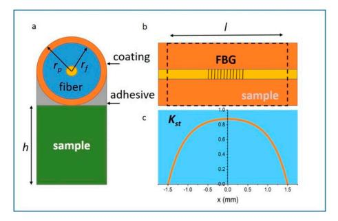
**Figure 11.** Schematics of a model to estimate the strain transfer (**a**) Cross-section of fiber plus sample ensemble for strain measurement. Here *h* is the sample thickness,  $r_p$  is the coating radius,  $r_f$  is the fiber cladding radius. (**b**) Fiber top view, indicating the sample length *l*, with respect to FBG position. (**c**) Strain transfer coefficient  $K_{st}$  plotted as a function of position *x* on the fiber, computed using Equation (3) with parameters in Table 1.
