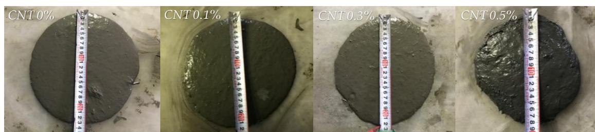
**Figure 6.** Flow table test results.
