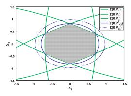
**Figure 12.** Illustration of three ellipsoids  $\varepsilon(0, P_1)$ ,  $\varepsilon(0, P_2)$ ,  $\varepsilon(0, P_3)$  and their fusion result  $\varepsilon(0, P_{CI})$ , provided by CI method. The figure also shows the actual fused result  $\varepsilon(0, P_{CI}^A)$  for CI.
