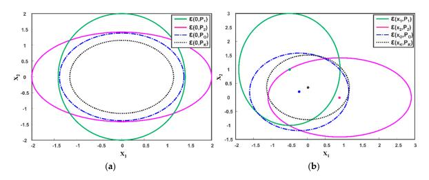
**Figure 5.** Ellipsoidal Fusion of two Estimates  $\varepsilon(x_1, P_1)$  and  $\varepsilon(x_2, P_2)$  (a) Zero Mean (b) Non-Zero Mean. Compared to the optimal solution  $\varepsilon(x_o, P_o)$ , Kalman filter (KF) yields underestimated results  $\varepsilon(x_K, P_K)$  by ignoring cross-correlation.
