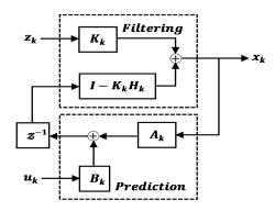
**Figure 4.** Kalman filter Prediction-Update procedure ( $z^{-1}$  represents a unit time delay).
