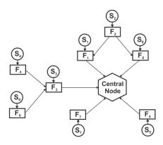
Figure 2. Distributed fusion architecture. Each node consists of sensor and fusion node.
