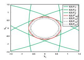
**Figure 13.** Illustration of three ellipsoids  $\varepsilon(0, P_1)$ ,  $\varepsilon(0, P_2)$ ,  $\varepsilon(0, P_3)$  and their fusion result provided by ME methods. The figure also shows the actual fused result  $\varepsilon(0, P_{ME}^A)$  for ME methods.
