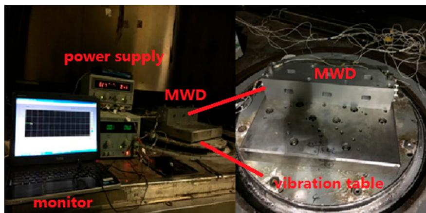
Figure 1. Vibration experiment setup.
