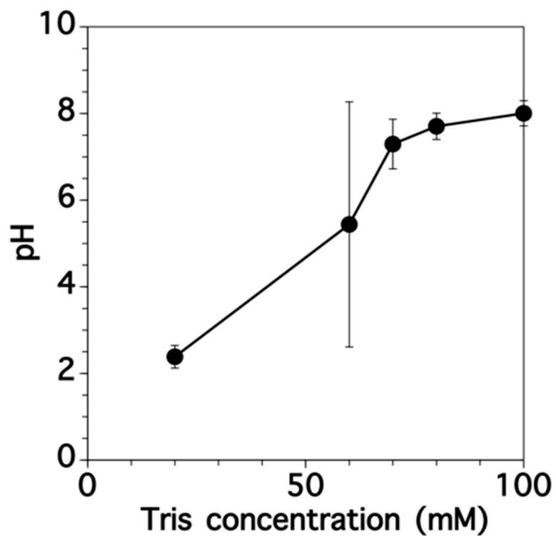
Figure S2. Effect of Tris concentration of the buffer solution on the pH of the solution under analysis.
