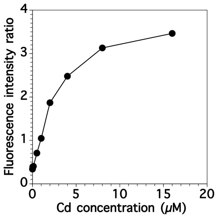
Figure S1. Calibration curve for Cd by fluorescence spectroscopy.
