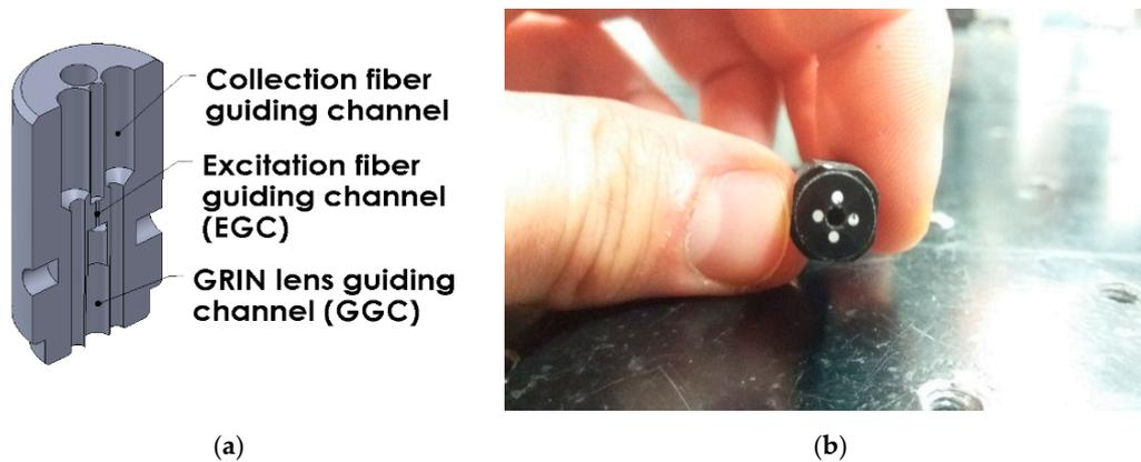
**Figure 2.** Fiber sensor head cross section (a) and a photograph of the sensor detection face (b). In the picture of the sensor face, the central part is a hole for the GRIN lens, while the four smaller circles surrounding it are collection fiber faces. The sensor's outer diameter is  $10 \pm 0,05$  mm. Sensors head was fabricated in the university CNC (Computerized Numerical Control) center.
