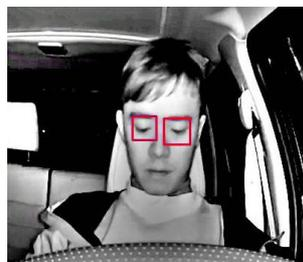
**Figure 5.** Failure to detect pupils.
