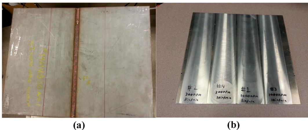
**Figure 5.** (a) A 12.7 mm thick 304 stainless steel plate; and (b) a 3 mm thick 2024 aluminum plate having four different degrees of surface roughness.
