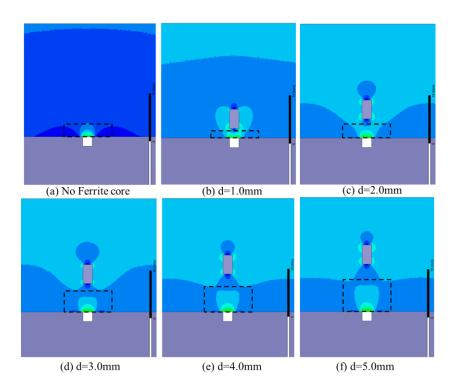
Figure 5. The distributions of the MFL affected by the ferrite core at different lift-off distances.
