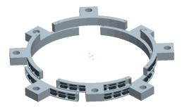
Figure 12. The MFL probing system integrated eight probes in two layers.
