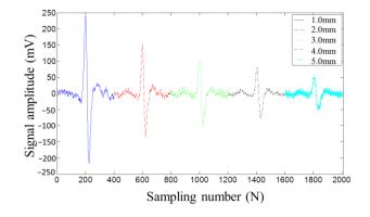
Figure 9. The MFL signals picked up by the lift-off-tolerant MFL sensor at different lift-off distances.
