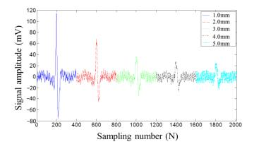
Figure 8. The MFL signals picked up by the induction coil at different lift-off distances.
