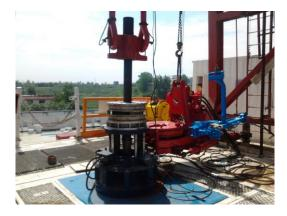
Figure 15. The whole MFL testing apparatus at the wellhead.
