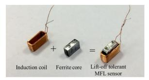
Figure 6. The diagram of the lift-off-tolerant MFL sensor.
