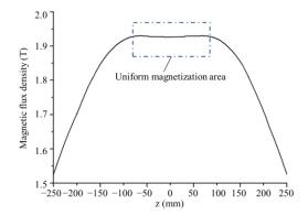
Figure 2. The axial magnetic flux density distribution in the drill pipe wall.
