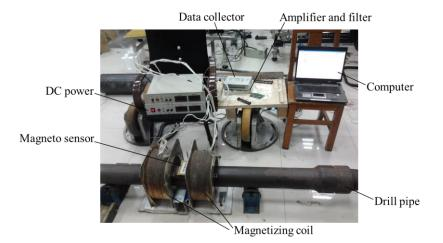
Figure 7. The experiment setup of the lift-off-tolerant MFL probe for drill pipes.
