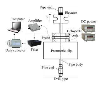
Figure 3. The diagram of the MFL (magnetic flux leakage) method for drill pipes at the wellhead.
