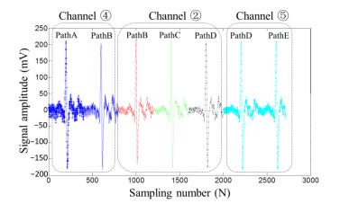
Figure 11. The MFL signals picked up by array lift-off-tolerant MFL sensors in different scanning paths.
