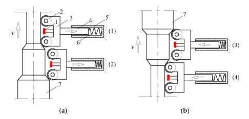
**Figure 13.** The follow-up scheme for the lift-off-tolerant MFL probing system. 1: probe; 2: wheel; 3: support; 4: slide; 5: guide rail; 6: pressure string; 7: pipe end. (**a**) the wheel rolling up the pipe end from Position (1) to Position (2); (**b**) the wheel rolling down the pipe end from Position (3) to Position (4).
