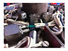
Figure 14. The lift-off-tolerant MFL probing system.
