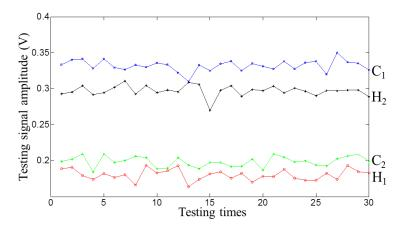
Figure 18. The testing signal amplitudes with the defects passed in different paths.
