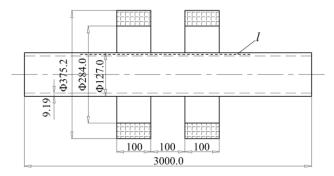
Figure 1. The simulation model for the 5 in. drill pipe magnetized by the Helmholtz coil (unit: mm).
