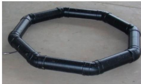
**Figure 12.** Experimental model of the AEM sensor.
