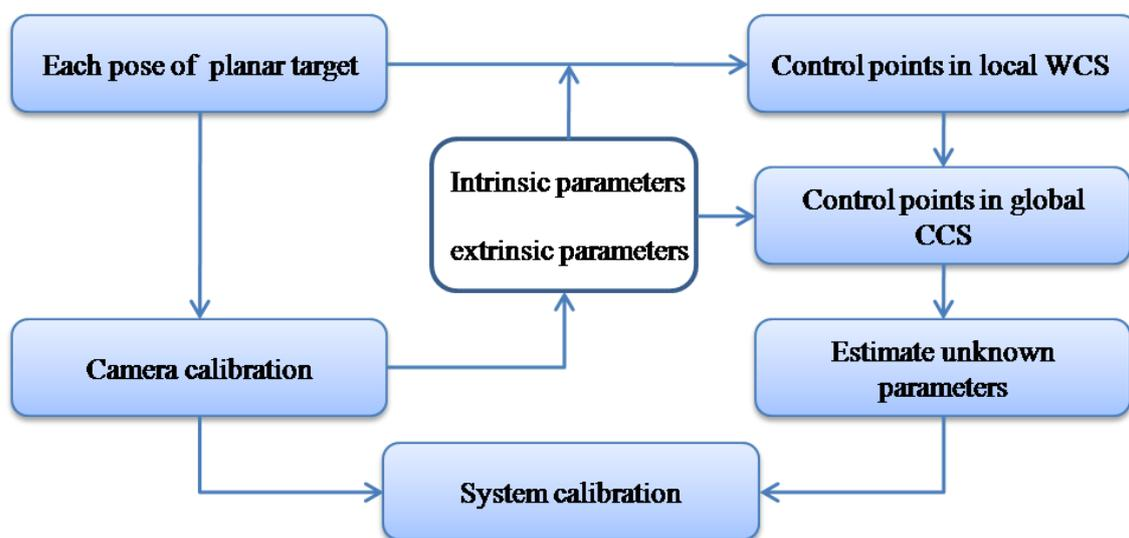
Figure 5. Flowchart of the one-mirror galvanometric laser scanner calibration procedures.
