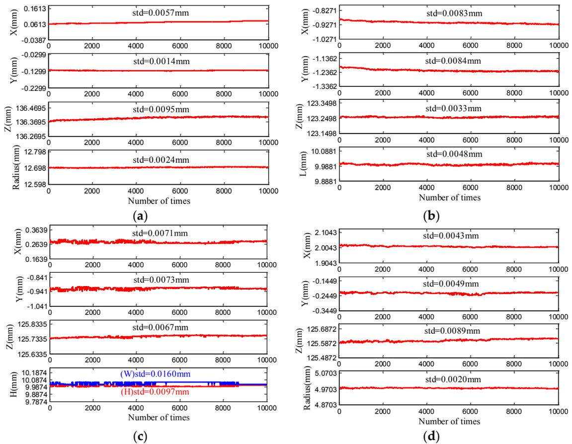
**Figure 8.** Repeatability evaluation of four features. (a) Sphere feature; (b) Slot feature; (c) Square feature; (d) Circle feature.
