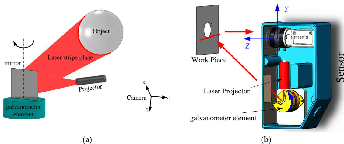
**Figure 1.** (a) Schematic diagram of the one-mirror galvanometric laser scanner; and (b) construction of the one-mirror galvanometric laser scanner.
