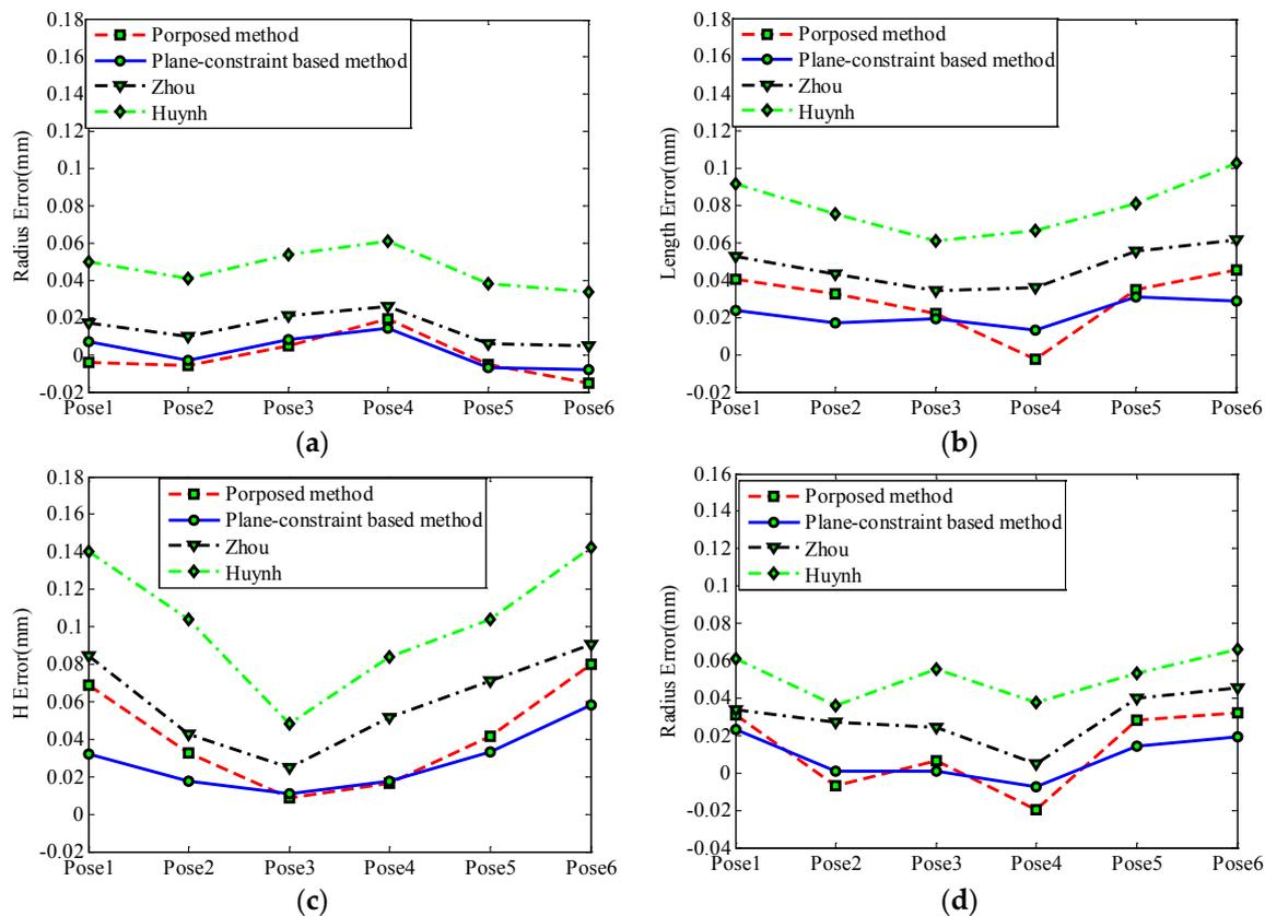
**Figure 9.** Accuracy comparison among four methods. (a) Sphere feature; (b) Slot feature; (c) Square feature; (d) Circle feature.
