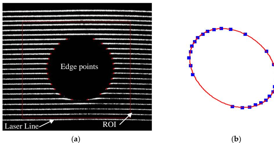
**Figure 2.** The measuring process of the work piece feature: (a) the processed gray image; and (b) the corresponding 3D point cloud.
