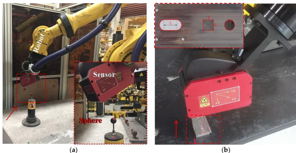
**Figure 6.** (a) The experimental setup in the automobile production line; and (b) the experimental setup in the laboratory condition.
