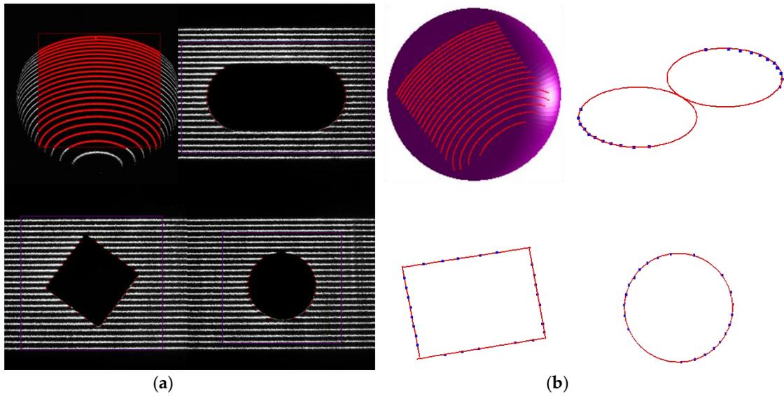
**Figure 7.** The measuring process of four features: (a) the processed gray image; and (b) the fitted four features.
