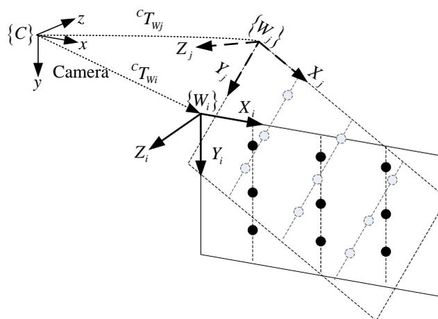
**Figure 3.** The diagrammatic sketch of transforming the multiple local world coordinate systems into a global camera coordinate system.
