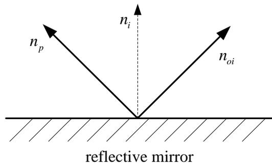
**Figure 4.** Schematic diagram of determining the reflected laser plane's normal vector.
