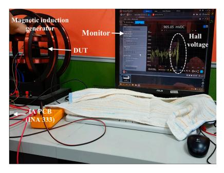
**Figure 7.** Hall voltage appears on the monitor evidently when the magnetic body comes in contact with the distance detector.
