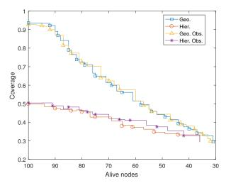
Figure 14. Coverage vs. number of nodes alive in an MWSN deployed with the proposed algorithm.
