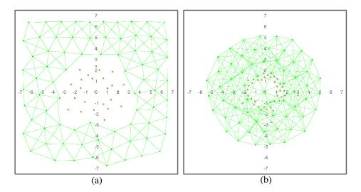
**Figure 3.** MWSN with geographic routing: (**a**) without clustering force; (**b**) with clustering force (figures are scaled 1:10 m).
