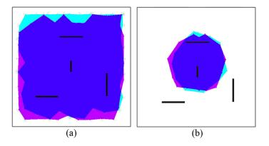
**Figure 9.** Deployment with geographic routing: area difference with and without obstacles: (**a**) initial; (**b**) final.
