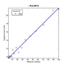
Figure 6. Power consumption vs. distance for CC2500 per packed transmitted.
