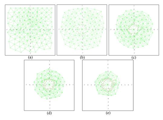
**Figure 7.** Network configuration when: (**a**) 0%; (**b**) 12.5%; (**c**) 25%; (**d**) 50% and (**e**) 70% of the nodes are dead (figures are scaled 1:10 m).
