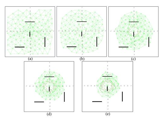
**Figure 8.** Network configuration when: (**a**) 0%; (**b**) 12.5%; (**c**) 25%; (**d**) 50% and (**e**) 70% of the nodes are dead (figures are scaled 1:10 m).
