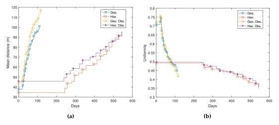
Figure 15. Node distribution evolution in time: (a) mean distance per (living) node; (b) network uniformity.
