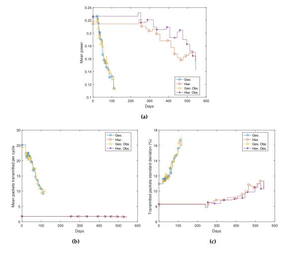
**Figure 16.** Power evolution in time: (**a**) mean power in the network; (**b**) mean transmitted packets; (**c**) transmitted packets' standard deviation.
