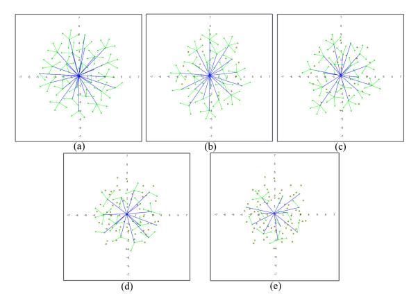
**Figure 10.** Network configuration when: (**a**) 0%; (**b**) 12.5%; (**c**) 25%; (**d**) 50% and (**e**) 70% of the nodes are dead (figures are scaled 1:10 m).
