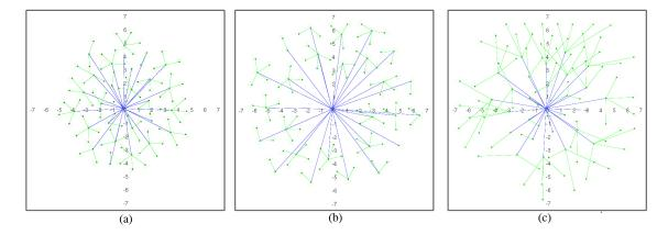
**Figure 4.** Hierarchical MWSN: (**a**) with all clustering forces; (**b**) without clustering force L1 vs. the sink node (L2); (**c**) without clustering force L0 vs. L1 (figures are scaled 1:10 m).
