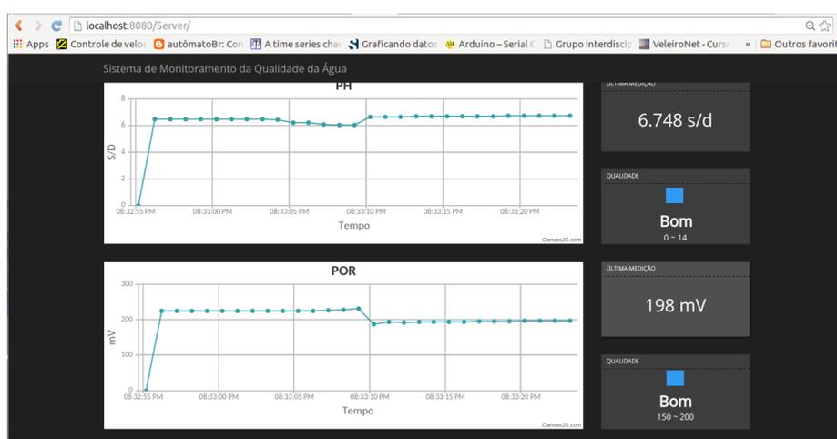
**Figure 16.** The web interface implemented for showing data on the Internet (already running at [www.natalnet.br/nboat](http://www.natalnet.br/nboat)).
