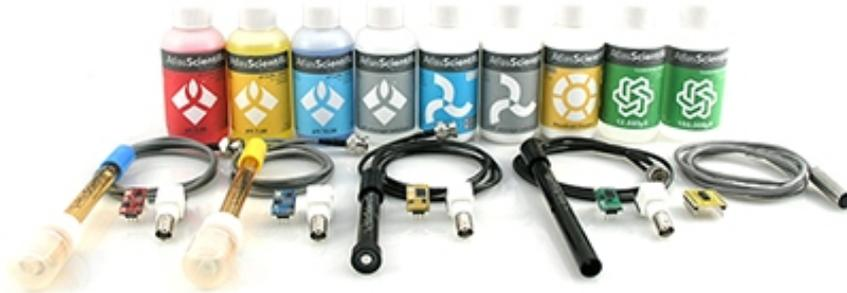
**Figure 1.** Kit of sensors adopted for water monitoring.
