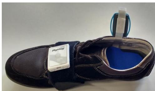
**Figure 1.** Instrumented shoe system (right shoe). The Physilog<sup>®</sup> is placed on a strap looping around the shoe with Velcro<sup>®</sup> tape. The insole (in blue) is placed inside the shoe and linked to the Physilog<sup>®</sup> by a cable. Converting electronics are in the box with handles (lateral side of the shoe), connected to the strip stemming from the insole.
