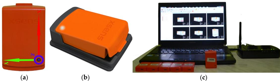
**Figure 2.** (a) MTw sensor unit; (b) Sensor unit with housing [26]; (c) Wireless data acquisition system.
