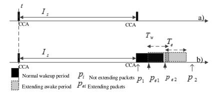
**Figure 3.** Low power listening protocol (LPL) operations: (**a**) CCA checks and (**b**) CCA checks with received packets.
