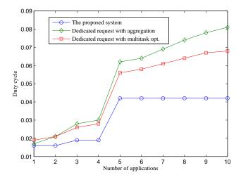
**Figure 5.** Average duty cycle vs. the number of applications that request sensing intervals as follows: 60 s, 120 s, 30 s, 40 s, 2 s, 5 s, 10 s, 15 s, 20 s and 25 s, respectively.
