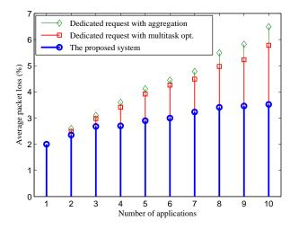
Figure 8. Average packet loss ratio vs. the number of applications.
