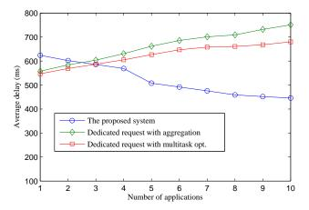
Figure 7. Average packet delivery delay vs. the number of applications.
