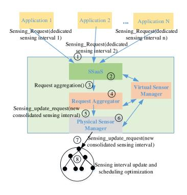
Figure 2. The proposed interactive model for the sensor-cloud.
