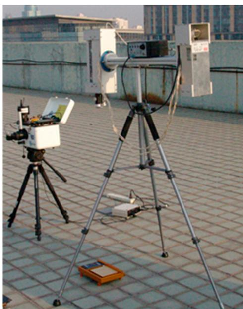
**Figure 2.** Air-cooling 10.6 μm CO<sub>2</sub> laser source and the 102F FTIR spectrometer.
