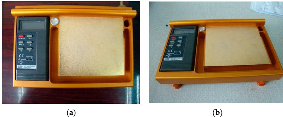
**Figure 3.** Photos of the diffuse reflecting gilded plate with steady-temperature water troughs.
