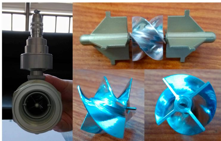
Figure 3. The DN20 turbine flow sensor picture.
