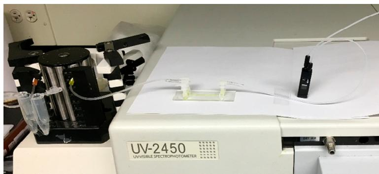
**Figure S4.** A different view of the experimental setup that was used to analyze the signal transduction process. The flow of solution was controlled by a Gilson MINIPULS<sup>®</sup> 3, which was used to push solution through the enzymatic flow cell and then into the flow-through cuvette before being discharged into a waste beaker. In this illustration, the flow through cuvette has been plumbed into the system, to illustrate the process.
