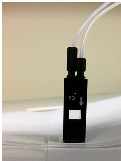
**Figure S5.** The commercial flow-cuvette connected to the tubing of the flow system. During the measurements the cuvette was placed inside the spectrophotometer.
