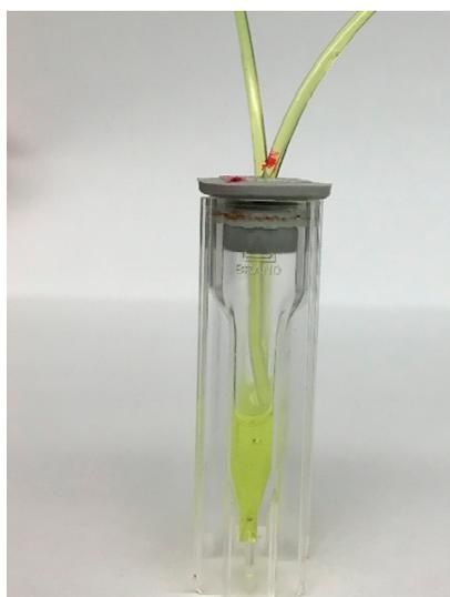
**Figure S6.** The lab-made flow-cuvette, please note that the volume of solution in the lab-made cuvette is tunable by adjusting the height of the outflow hose. In this illustration, dye is used to make the height of solution visible. During the measurements the cuvette was placed inside the spectrophotometer.
