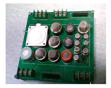
Figure 1. Electronic nose sensor array.
