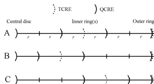
**Figure 5.** Relative locations of rings, with respect to the central disc, for constant inter-ring distances (A), increasing inter-ring distances (B), and decreasing inter-ring distances (C) TCRE and QCRE configurations.
