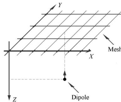
**Figure 4.** Schematic of the FEM model with an evenly spaced square mesh size of  $600 \times 600$  used to assess and compare the accuracy of Laplacian estimates for constant and variable inter-ring distances CRE configurations.
