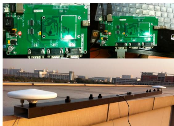
Figure 10. Receiver electric circuit and antennae configuration.
