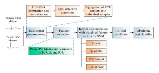
Figure 1. Classifier development flow of electrocardiogram drunk driving detection (ECG-DDD).
