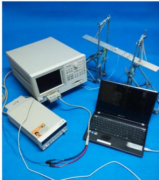
**Figure 3.** Experimental setup for impedance measurements on the bolt-jointed aluminium beam.
