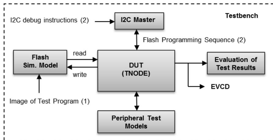
Figure 5. TNODE5 testbench: (1) Test execution from Flash; (2) Test execution via I<sup>2</sup>C debug port.
