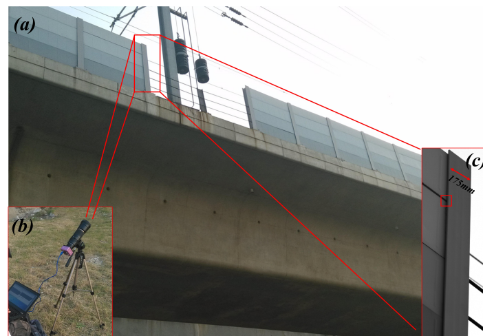
Figure 11. Sound barrier experiment setup: (a) the experiment environment; (b) experimental setup; (c) Image captured by the developed visual measuring system.
