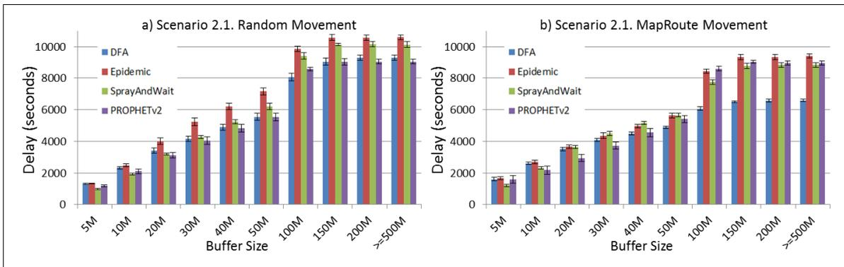
**Figure 26.** Results for scenario 2.1. Average delay in seconds with different Buffer Sizes, generating 2 MB messages every 1 to 2 min, (a) MAPs moving randomly on the path; (b) MAPs following the path in only one direction. DFA: Distributed Forwarding Algorithm.
