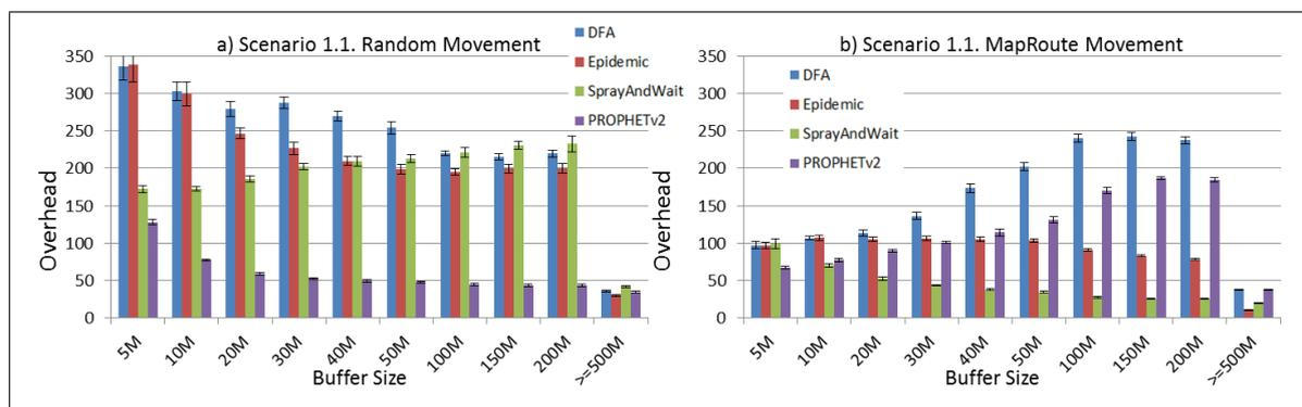
**Figure 12.** Results for scenario 1.1. Average overhead with different Buffer Sizes, generating 2 MB messages every 1 to 2 min, (a) MAPs moving randomly on the path; (b) MAPs following the path in only one direction. DFA: Distributed Forwarding Algorithm.
