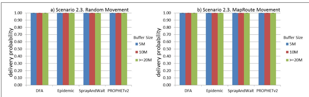
**Figure 33.** Results for scenario 2.3. Delivery probabilities with different Buffer Sizes, generating 2 kB messages every 1 to 2 h, (a) MAPs moving randomly on the path; (b) MAPs following the path in only one direction. DFA: Distributed Forwarding Algorithm.
