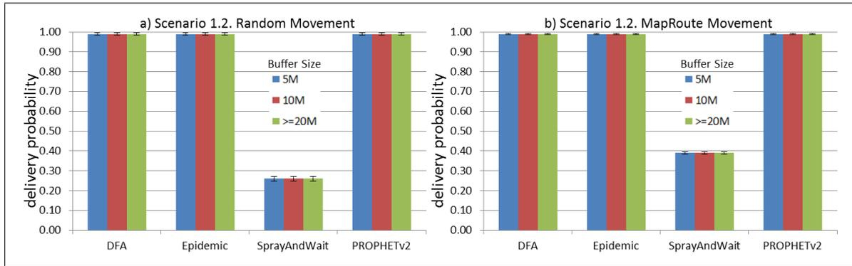
**Figure 13.** Results for scenario 1.2. Delivery probabilities with different Buffer Sizes, generating 2 kB messages every 1 to 2 min, (a) MAPs moving randomly on the path; (b) MAPs following the path in only one direction. DFA: Distributed Forwarding Algorithm.
