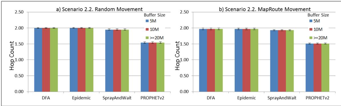
**Figure 31.** Results for scenario 2.2. Average hop count with different Buffer Sizes, generating 2 kB messages every 1 to 2 min, (a) MAPs moving randomly on the path; (b) MAPs following the path in only one direction. DFA: Distributed Forwarding Algorithm.
