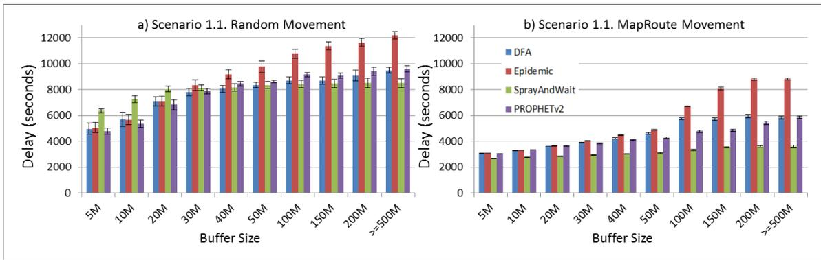
**Figure 10.** Results for scenario 1.1. Average delay in seconds with different Buffer Sizes, generating 2 MB messages every 1 to 2 min, (a) MAPs moving randomly on the path; (b) MAPs following the path in only one direction. DFA: Distributed Forwarding Algorithm.
