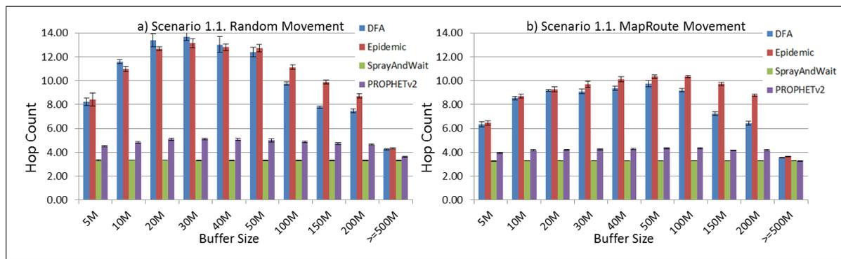
**Figure 11.** Results for scenario 1.1. Average hop count with different Buffer Sizes, generating 2 MB messages every 1 to 2 min, (a) MAPs moving randomly on the path; (b) MAPs following the path in only one direction. DFA: Distributed Forwarding Algorithm.
