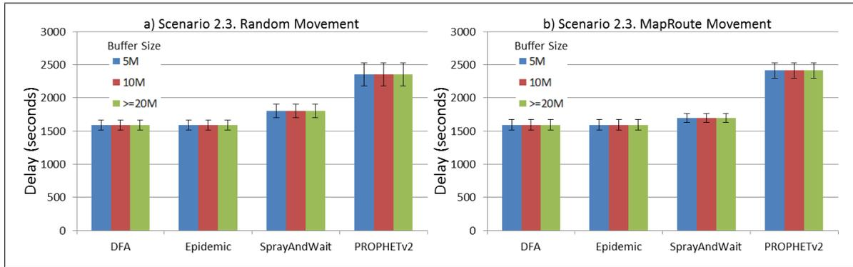
**Figure 34.** Results for scenario 2.3. Average delay in seconds with different Buffer Sizes, generating 2 kB messages every 1 to 2 h, (a) MAPs moving randomly on the path; (b) MAPs following the path in only one direction. DFA: Distributed Forwarding Algorithm.
