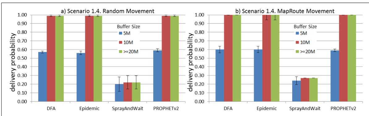
**Figure 21.** Results for scenario 1.4. Delivery probabilities with different Buffer Sizes, generating 2 MB messages every 1 to 2 h, (a) MAPs moving randomly on the path; (b) MAPs following the path in only one direction. DFA: Distributed Forwarding Algorithm.
