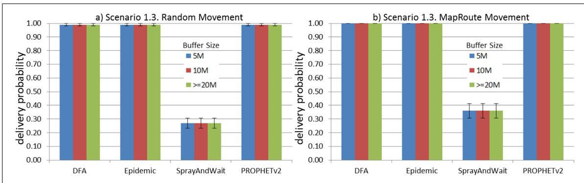
**Figure 17.** Results for scenario 1.3. Delivery probabilities with different Buffer Sizes, generating 2 kB messages every 1 to 2 h, (a) MAPs moving randomly on the path; (b) MAPs following the path in only one direction. DFA: Distributed Forwarding Algorithm.
