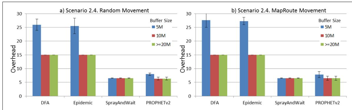
**Figure 40.** Results for scenario 2.4. Average overhead with different Buffer Sizes, generating 2 MB messages every 1 to 2 h, (a) MAPs moving randomly on the path; (b) MAPs following the path in only one direction. DFA: Distributed Forwarding Algorithm.
