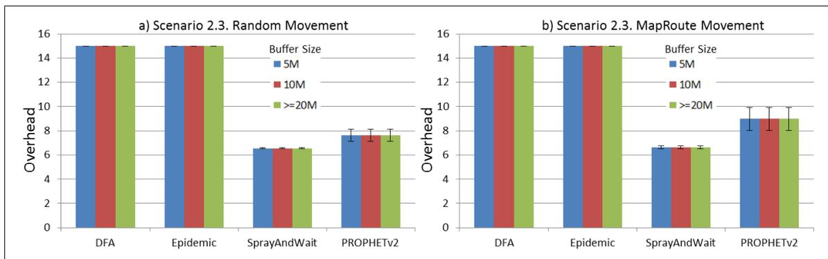
**Figure 36.** Results for scenario 2.3. Average overhead with different Buffer Sizes, generating 2 kB messages every 1 to 2 h, (a) MAPs moving randomly on the path; (b) MAPs following the path in only one direction. DFA: Distributed Forwarding Algorithm.
