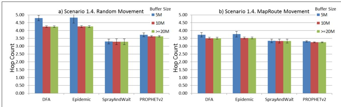
**Figure 23.** Results for scenario 1.4. Average hop count with different Buffer Sizes, generating 2 MB messages every 1 to 2 h, (a) MAPs moving randomly on the path; (b) MAPs following the path in only one direction. DFA: Distributed Forwarding Algorithm.
