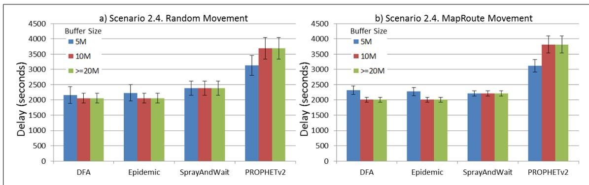
**Figure 38.** Results for scenario 2.4. Average delay in seconds with different Buffer Sizes, generating 2 MB messages every 1 to 2 h, (a) MAPs moving randomly on the path; (b) MAPs following the path in only one direction. DFA: Distributed Forwarding Algorithm.
