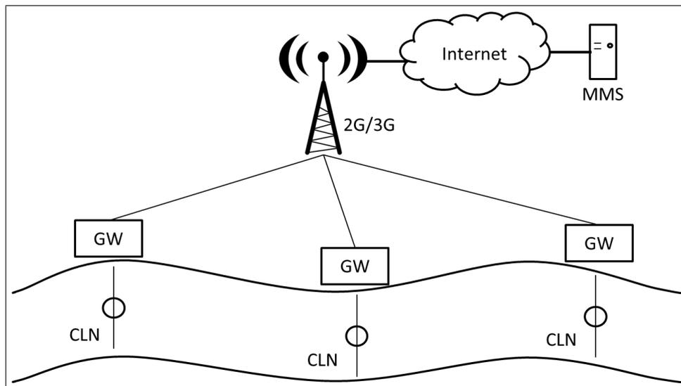
**Figure 1.** GOLDFISH project description. Sensor Nodes (CLN), Management and Monitoring Station (MMS), and Gateways (GW) are depicted.
