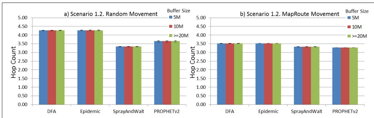
**Figure 15.** Results for scenario 1.2. Average hop count with different Buffer Sizes, generating 2 kB messages every 1 to 2 min, (a) MAPs moving randomly on the path; (b) MAPs following the path in only one direction. DFA: Distributed Forwarding Algorithm.
