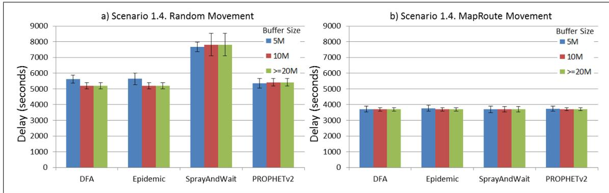
**Figure 22.** Results for scenario 1.4. Average delay in seconds with different Buffer Sizes, generating 2 MB messages every 1 to 2 h, (a) MAPs moving randomly on the path; (b) MAPs following the path in only one direction. DFA: Distributed Forwarding Algorithm.
