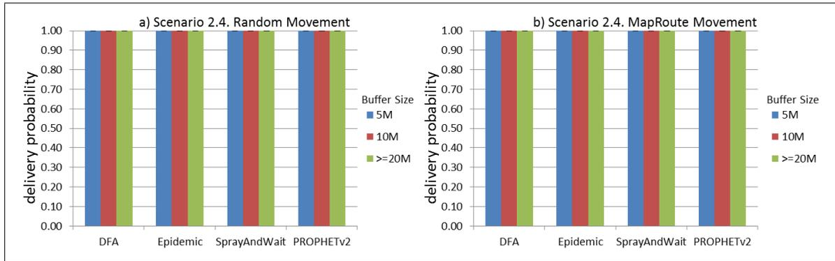
**Figure 37.** Results for scenario 2.4. Delivery probabilities with different Buffer Sizes, generating 2 MB messages every 1 to 2 h, (a) MAPs moving randomly on the path; (b) MAPs following the path in only one direction. DFA: Distributed Forwarding Algorithm.
