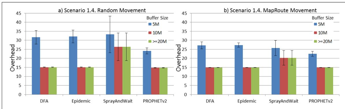
**Figure 24.** Results for scenario 1.4. Average overhead with different Buffer Sizes, generating 2 MB messages every 1 to 2 h, (a) MAPs moving randomly on the path; (b) MAPs following the path in only one direction. DFA: Distributed Forwarding Algorithm.
