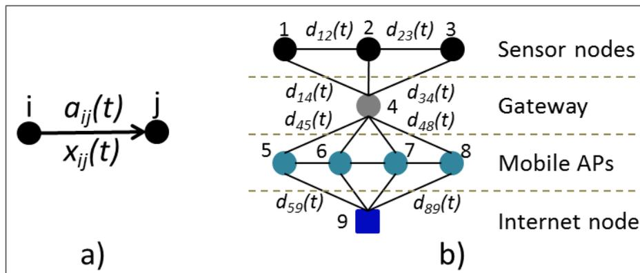
**Figure 4.** Problem graph. (a) Availability probability and data flow from node  $i$  to node  $j$ ; (b) Network graph with delivery probabilities varying through time. AP: Access Point.
