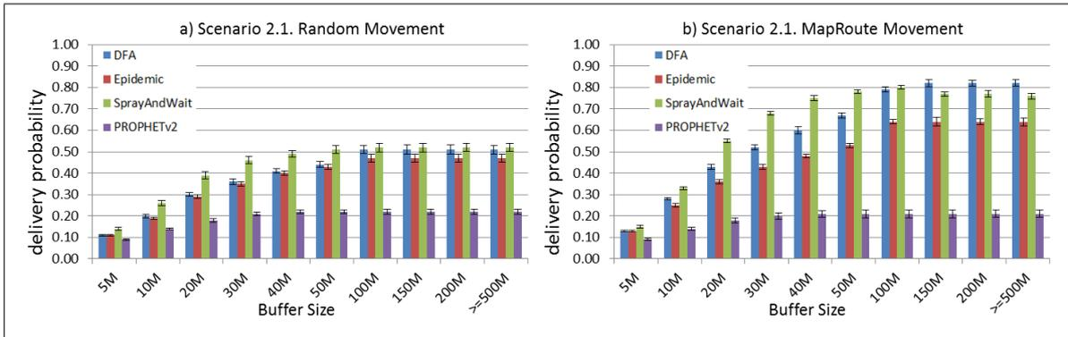
**Figure 25.** Results for scenario 2.1. Delivery probabilities with different Buffer Sizes, generating 2 MB messages every 1 to 2 min, (a) MAPs moving randomly on the path; (b) MAPs following the path in only one direction. DFA: Distributed Forwarding Algorithm.
