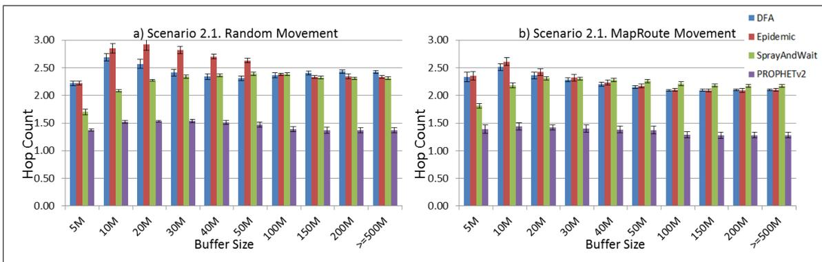
**Figure 27.** Results for scenario 2.1. Average hop count with different Buffer Sizes, generating 2 MB messages every 1 to 2 min, (a) MAPs moving randomly on the path; (b) MAPs following the path in only one direction. DFA: Distributed Forwarding Algorithm.
