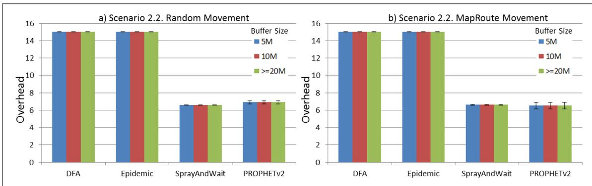
**Figure 32.** Results for scenario 2.2. Average overhead with different Buffer Sizes, generating 2 kB messages every 1 to 2 min, (a) MAPs moving randomly on the path; (b) MAPs following the path in only one direction. DFA: Distributed Forwarding Algorithm.
