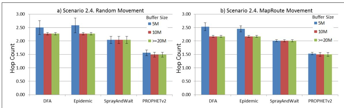
**Figure 39.** Results for scenario 2.4. Average hop count with different Buffer Sizes, generating 2 MB messages every 1 to 2 h, (a) MAPs moving randomly on the path; (b) MAPs following the path in only one direction. DFA: Distributed Forwarding Algorithm.
