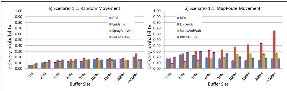
**Figure 9.** Results for scenario 1.1. Delivery probabilities with different Buffer Sizes, generating 2 MB messages every 1 to 2 min, (a) MAPs moving randomly on the path. (b) MAPs following the path in only one direction. DFA: Distributed Forwarding Algorithm.
