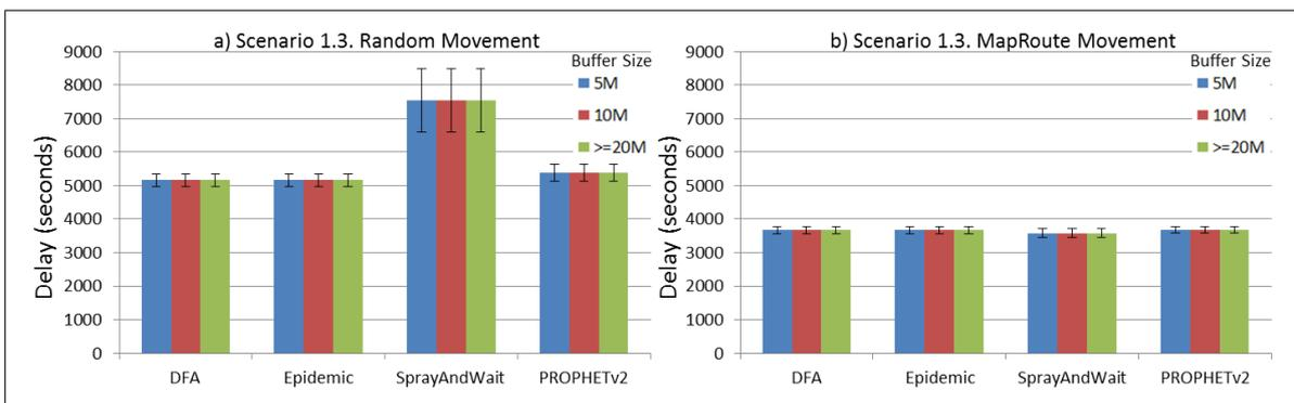
**Figure 18.** Results for scenario 1.3. Average delay in seconds with different Buffer Sizes, generating 2 kB messages every 1 to 2 h, (a) MAPs moving randomly on the path; (b) MAPs following the path in only one direction. DFA: Distributed Forwarding Algorithm.
