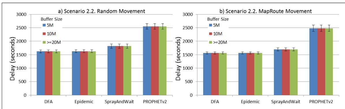
**Figure 30.** Results for scenario 2.2. Average delay in seconds with different Buffer Sizes, generating 2 kB messages every 1 to 2 min, (a) MAPs moving randomly on the path; (b) MAPs following the path in only one direction. DFA: Distributed Forwarding Algorithm.
