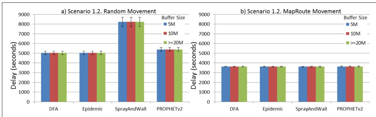
**Figure 14.** Results for scenario 1.2. Average delay in seconds with different Buffer Sizes, generating 2 kB messages every 1 to 2 min, (a) MAPs moving randomly on the path; (b) MAPs following the path in only one direction. DFA: Distributed Forwarding Algorithm.
