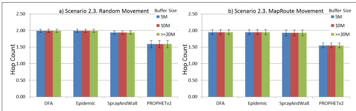
**Figure 35.** Results for scenario 2.3. Average hop count with different Buffer Sizes, generating 2 kB messages every 1 to 2 h, (a) MAPs moving randomly on the path; (b) MAPs following the path in only one direction. DFA: Distributed Forwarding Algorithm.
