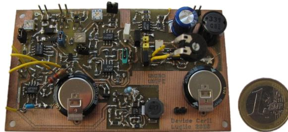
**Figure 10.** Picture of the assembled multi-source energy harvester. The wind energy harvesting section is on the rightmost side: from top downwards, the radial electrolytic capacitor  $C_1$ , the radial inductor  $L$ , the trimmer  $R_3$  and the supercapacitor  $C_2$  are clearly recognizable.
